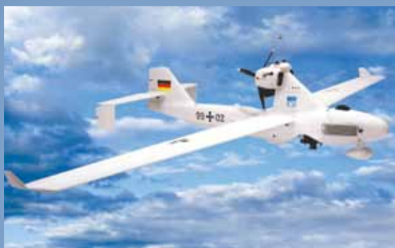
The unmanned reconnaissance drone Luna X-2000 sends video and data to a ground station in real-time. The German government has employed the lightweight craft in Iraq and Kosovo.
